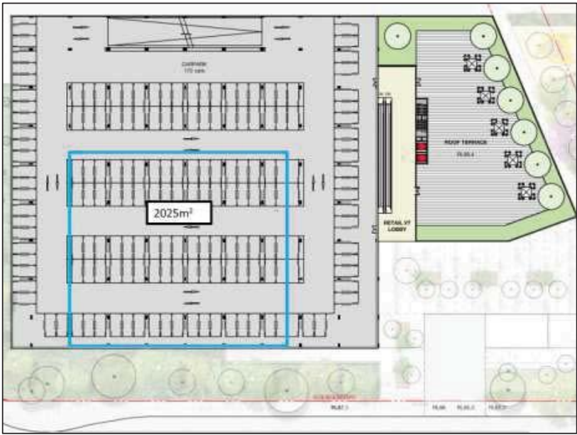
Figure 14 Indicative floorplate (in blue) of above ground parking with four levels and 344 spaces
